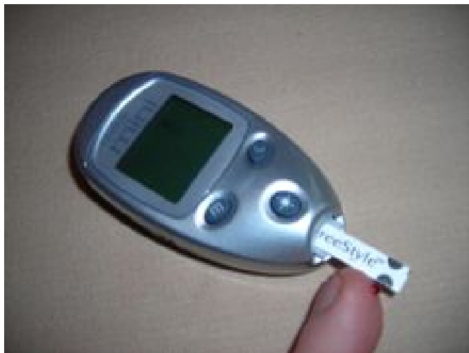
Figure 3: A person with diabetes has to monitor their blood glucose carefully. This glucose meter analyses only a small drop of blood. (Source: http://commons.wikimedia.org/wiki/Image:Glucose_test.jpg , License: GFDL 1.2)
